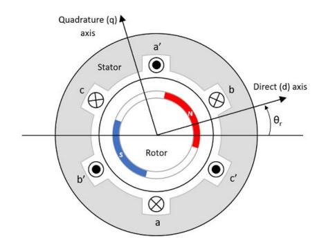
The motor magnetic field due to the permanent magnets creates a sinusoidal rate of change of flux with motor angle.
