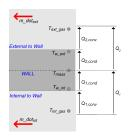
The block implements these equations to calculate the heat transfer,  $Q_1$ , from the internal control volume gas to the internal wall depth,  $D_{int\_cond}$ .
