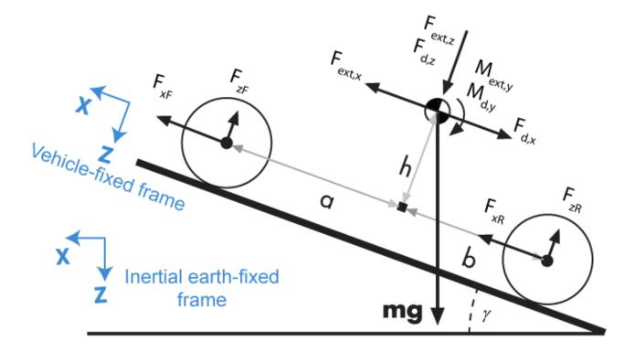
The Vehicle Body 1DOF Longitudinal block implements these equations.
