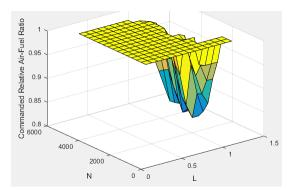
The block calculates the estimated fuel mass flow rate using the commanded lambda,  $\lambda_{cmd}$ , stoichiometric AFR, and estimated air mass flow rate.
