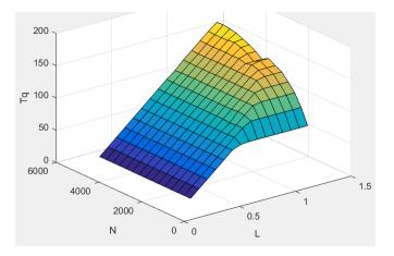
The simple torque lookup model assumes that the calibration has negative torque values to indicate the non-firing engine load (L) versus speed (N) condition. The calibrated table (L-by-N) contains the non-firing data in the first table row (1-by-N). When the fuel delivered to the engine is zero, the model uses the data in the first table row (1-by-N) at or above 100 AFR. 100 AFR results from fuel cutoff or very lean operation where combustion cannot occur.
