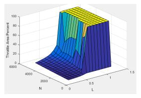
• To account for the non-linearity of the throttle position to throttle area, the throttle position percent lookup table linearizes the open-loop air mass flow control.
