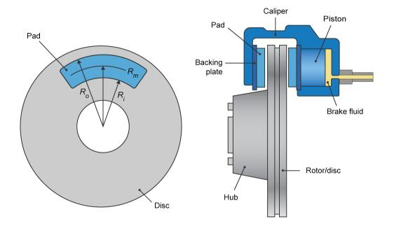
A disc brake converts brake cylinder pressure from the brake cylinder into force. The disc brake applies the force at the brake pad mean radius.
